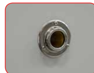
Side through hole of 25 mm diameter to install probes inside the chamber
