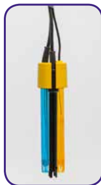
Electrode holder for field application with 3 holes
