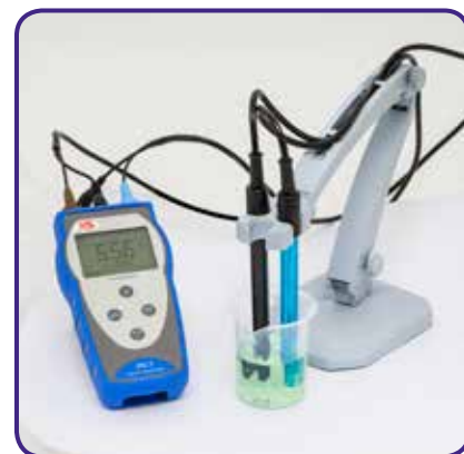
Electrode holder for use on laboratory bench (optional)
