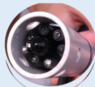
Multi Ion probe with 6 ISE, pH and temperature
