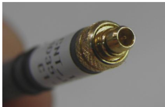
Detail of the mini-coaxial connector (electrode)
